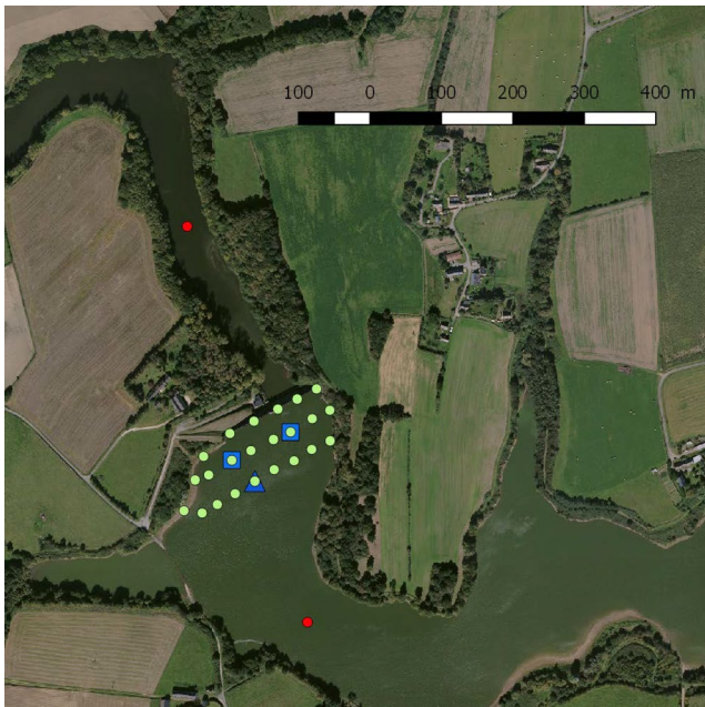
FIGURE 3 Location of the acoustic receivers with millisecond accuracy (green points) used to obtain accurate positions, and those without millisecond accuracy (red points) used to monitor the downstream or upstream movement of eels in Bois Joli Reservoir. Blue squares represent the location of the two test transmitters and blue triangle represents the position of the synchronization transmitter (ST) and reference receiver
