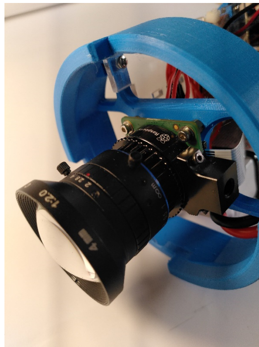
Figure 5. AICO lens with C-mount ring and Pi-Camera HQ 12MP secured on 3D-printed support.
