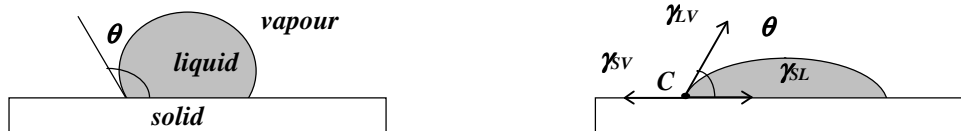
Figure 2: Contact angle ( \theta ) of a liquid droplet with the surface of a solid and thermodynamic equilibrium condition at the triple point C .
