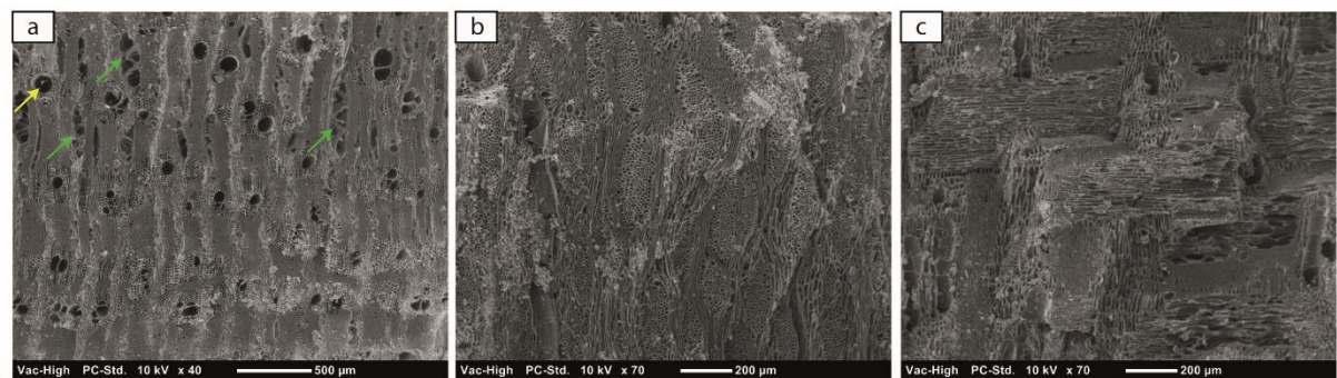
Figure 5. Acacia ehrenbergiana/etbaica/tortilis type. Transversal (a), tangential (b) and radial (c) sections (© C. Bouchaud). Green arrows = radial cracks; yellow arrow = fungi hyphae.
