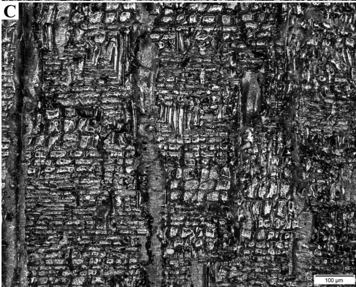
Fig. 2: A) TS: Vessels exclusively solitary, with mean diameter of lumina smaller than 50 \mu\text{m} . B) TLS: Short rays, 1- to 3 cells wide. Prismatic crystals in axial parenchyma cells. C) RLS: Body ray cells procumbent with 2-4 rows of upright and / or square marginal cells.
