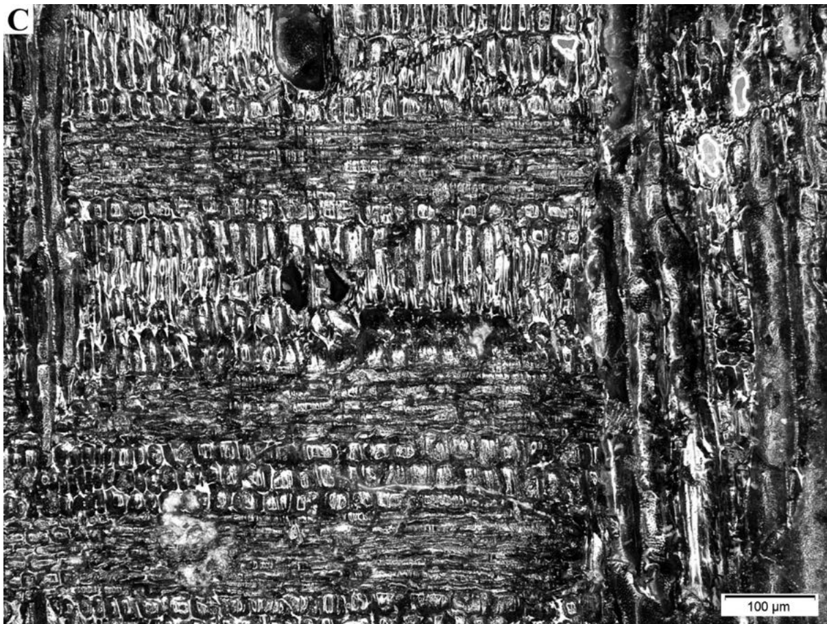
Fig. 9: A) TS: Vessels in diagonal and / or radial pattern with a mean diameter of lumina between 50-100 µm. Axial parenchyma paratracheal scanty to vasicentric. B) TLS: Ray width 1- to 3 cells, intervessel pits minute. C) RLS: Ray structure heterocellular.
